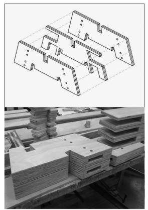
Fig. 4. Complex laminated plywood blocks.
