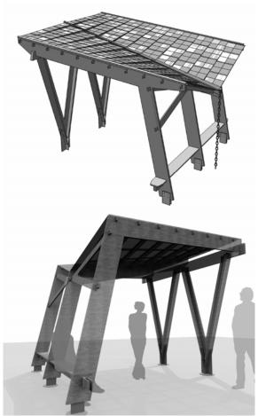
Fig. 3. First proposal (below) refined to add roof overhang and rain-chain (above).
